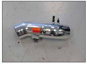
18. Install the provided NPT vent fittings into the  $K\&N^{\otimes}$  intake tube as shown.
