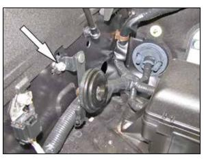
12. Remove the bolt which secures the horn to the inner fender.
