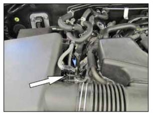
2. Disconnect the mass air sensor electrical connection and then unhook the wiring harness from the air box.
